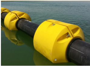
Pipelines for dredges and floats
