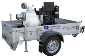
Trolley mounted pumps
